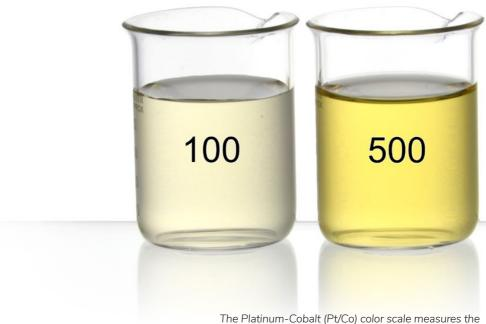
The Platinum-Cobalt (Pt/Co) color scale measures the "yellowness" of a liquid and is well suited for quality control and contamination detection.
