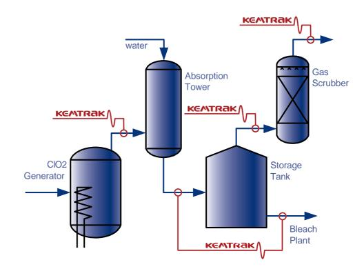
Optimize the reaction efficiency of ClO<sub>2</sub> generation, improve the control of vent-gas scrubbers to reduce atmospheric emissions and monitor the final concentration of ClO<sub>2</sub> sent to the bleaching plant.
