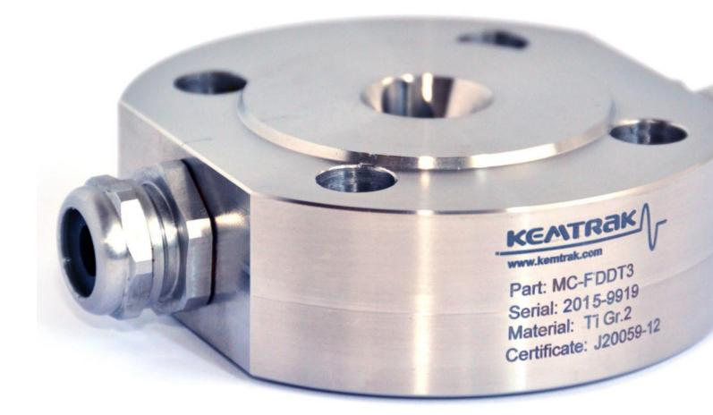
The Kemtrak DCP007 process photometer is used to optimize the efficiency of ClO<sub>2</sub> generation, improve the control of vent-gas scrubbers reducing atmospheric emissions and for monitoring the final concentration of ClO<sub>2</sub> sent to the bleaching plant. Robust corrosion resistant titanium measurement cells with sapphire windows and double o-ring sealing ensure a maintenance free operation.
