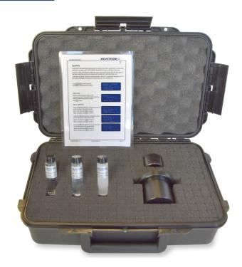
Each kit includes a vial holder specifically matched to the measurement cell, a light exclusion cap, and a set of three sealed calibration vials (20, 100, and 800 FTU). The sealed vials are ISO 7027 compliant and come with certification, ensuring traceability and regulatory compliance.
