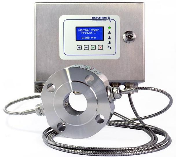
The [Kemtrak DCP007](#) process photometer has a high performance long life LED light source, precision optical filters and robust fiber optics that results in an ICUMSA color analyzer with outstanding performance and reliability.
