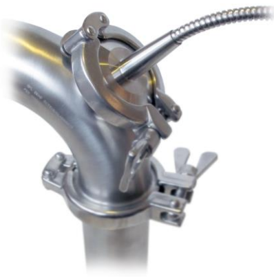
Kemtrak DN25/1" sanitary clamp pipe coupling fiber optic reflectance probe installed in a DN50/2" pipeline.
