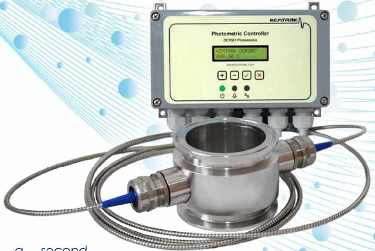
a second reference wavelength, which is not absorbed by the process medium, compensates for turbidity and/or fouling of the optical windows.
