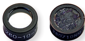
left: Optical filter used on a Kemtrak DCP007-UV photometer right: Eroded optical filter from a traditional hot mercury vapor lamp photometer
