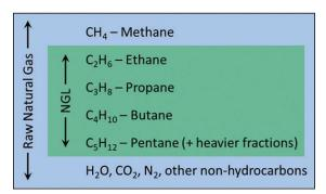
Gas processing plants separate methane (C1) from the raw natural gas stream for distribution around the country in natural gas pipelines. The remaining products (C2+) are typically transported in an NGL pipeline for further processing at other facilities such as refineries.
